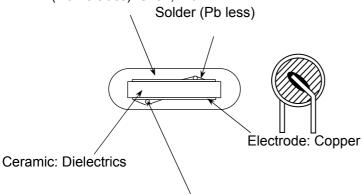
Lead wire: CP wire (Tin plated copper covers steel wire, Pb less)
