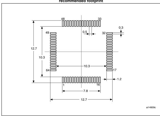
Figure 35. LQFP64 - 64-pin, 10 x 10 mm low-profile quad flat package recommended footprint
