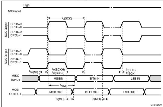
Figure 29. SPI timing diagram - master mode<sup>(1)</sup>
