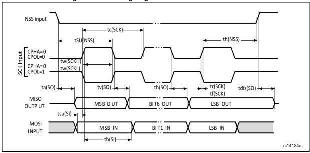
Figure 27. SPI timing diagram - slave mode and CPHA=0
