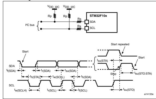
Figure 26. I<sup>2</sup>C bus AC waveforms and measurement circuit<sup>(1)</sup>
