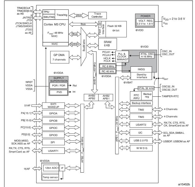
Figure 1. STM32F102T8 medium-density USB access line block diagram
