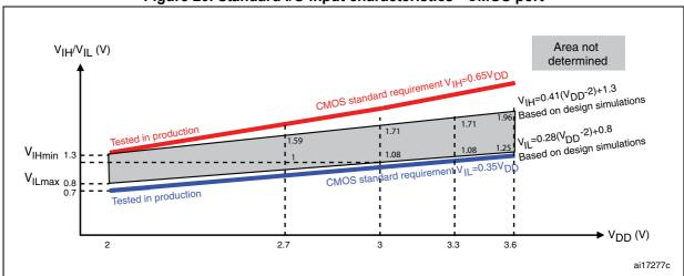
Figure 20. Standard I/O input characteristics - CMOS port
