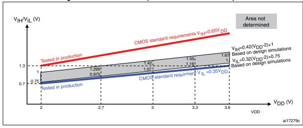
Figure 22. 5 V tolerant I/O input characteristics - CMOS port
