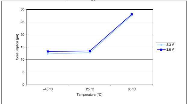
Figure 15. Typical current consumption in Standby mode versus temperature at  $V_{DD}$  = 3.3 V and 3.6 V
