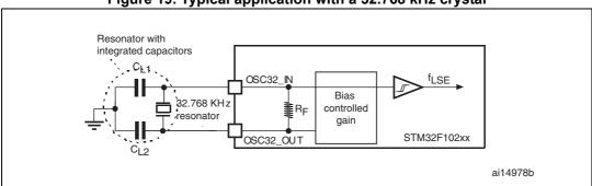
Figure 19. Typical application with a 32.768 kHz crystal
