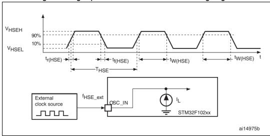
Figure 16. High-speed external clock source AC timing diagram
