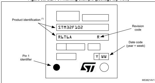
Figure 36. LQFP64 marking example (package top view)
