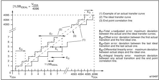
Figure 31. ADC accuracy characteristics
