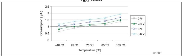
Figure 13. Typical current consumption in Stop mode with regulator in Run mode versus temperature at  $V_{DD}$  = 3.3 V and 3.6 V
