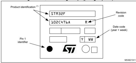
Figure 39. LQFP48 marking example (package top view)
