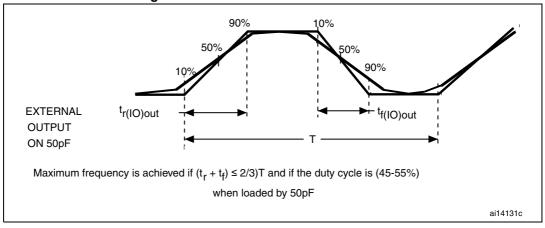
Figure 24. I/O AC characteristics definition
