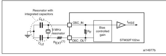
Figure 18. Typical application with an 8 MHz crystal
