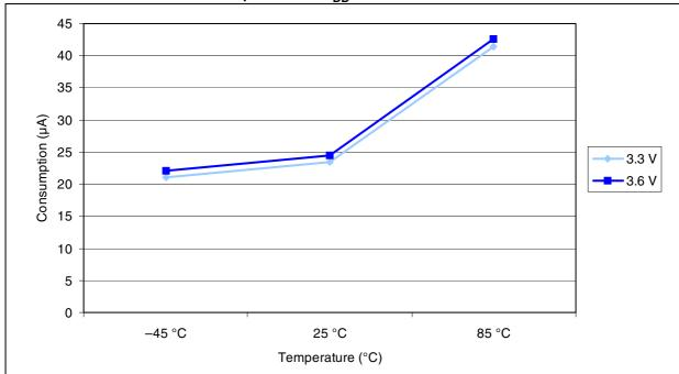
Figure 14. Typical current consumption in Stop mode with regulator in Low-power mode versus temperature at  $V_{DD}$  = 3.3 V and 3.6 V
