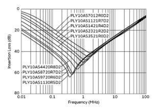
Common Mode Insertion Loss (Typ.)
