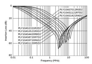
Differential Mode Insertion Loss (Typ.)
