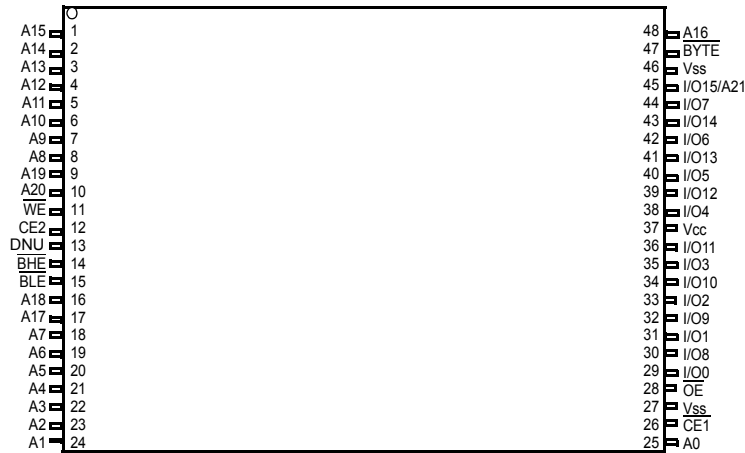
Figure 1. 48-pin TSOP I pinout (Front View) [1, 2]
