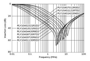
Differential Mode Insertion Loss (Typ.)
