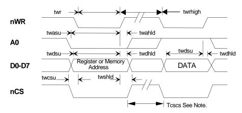
I/O Write Cycle to Register or Memory Buffer
