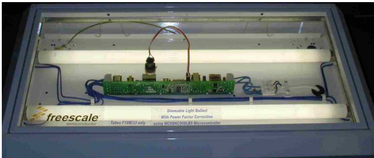
Figure 1-1. Dimmable Light Ballast with PFC Demo
